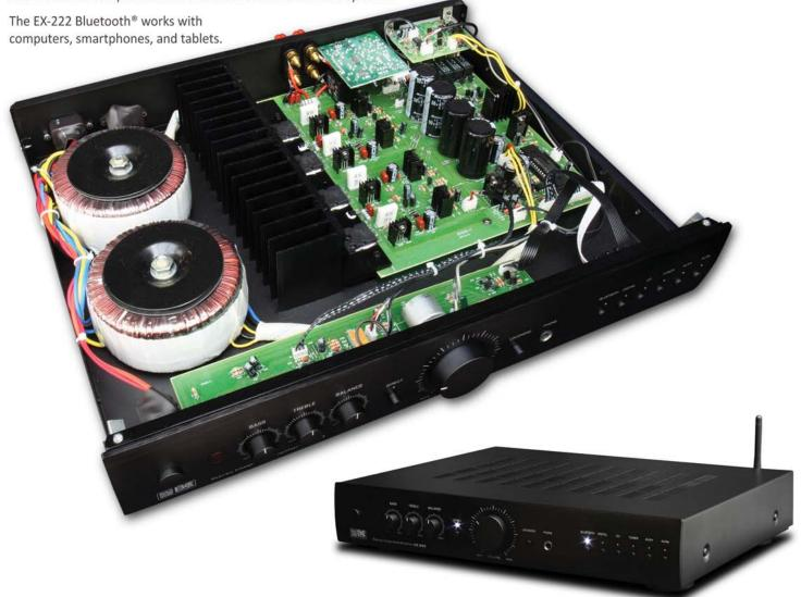
The EX-222 is dual power supply equipped, using two 200 VA Toroidal transformers. The amplifier stages share the same structure with famous EX-302, but with a doubled capacitive decoupling and a higher voltage level for final stages.
