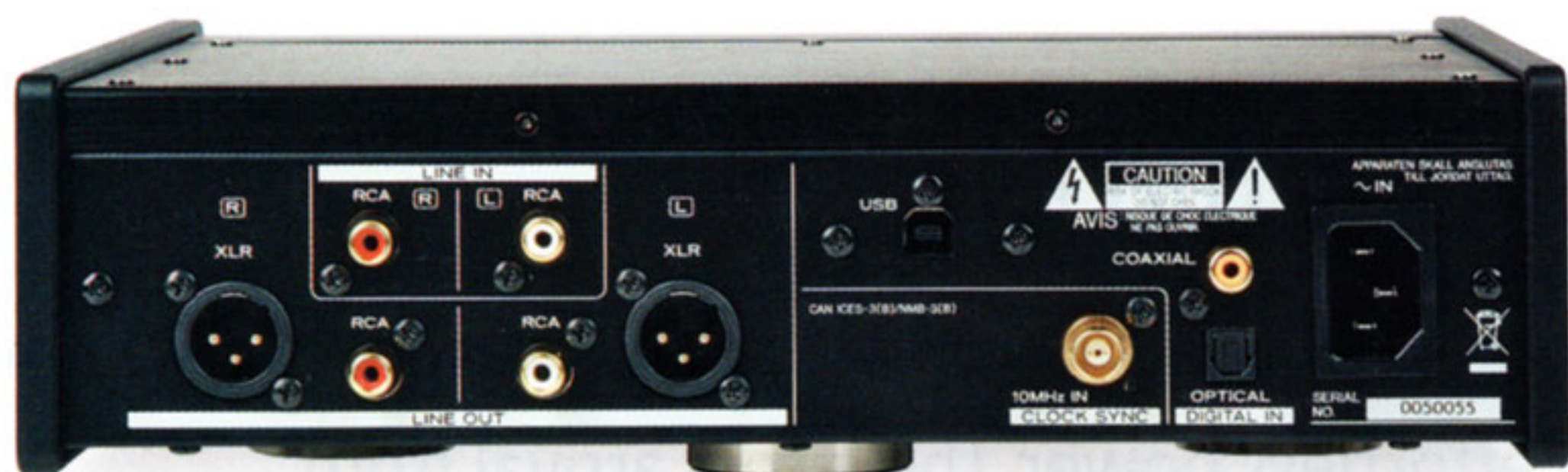
ABOVE: A standard set of digital ins is offered, including 384kHz/32-bit and DSD256 on USB, and 192kHz/24-bit S/PDIF on coax and optical. RCAs cover analogue ins and outs with XLRs for balanced outs, both fixed and variable with 0dB and +6dB options
